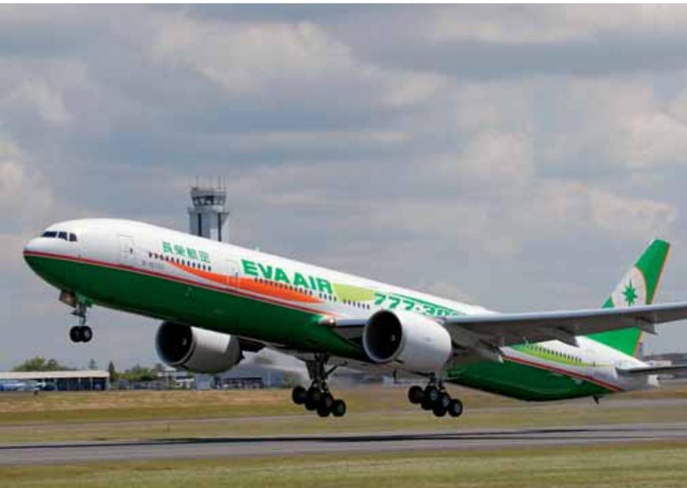
A review of this data shows that the A380 has the greatest net payload of 175,690lbs, although it is the 777-200LR that has the highest available structural payload for cargo at 74,400lbs (see table, page 35). However, the 777-300 and -300ER have the highest available container volume of 3,500 cubic feet, and so the highest belly freight capacities. The A340-600 has the second highest volume.
