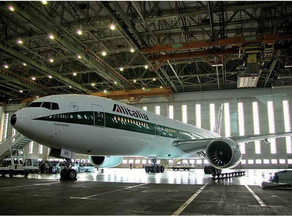
*777s that are used for long-haul operations generate 4,500-5,000FH per year in most cases. Most operators' maintenance programmes are a system of either annual or bi-annual base checks, with a heavy check being completed at an eight-year interval.*
