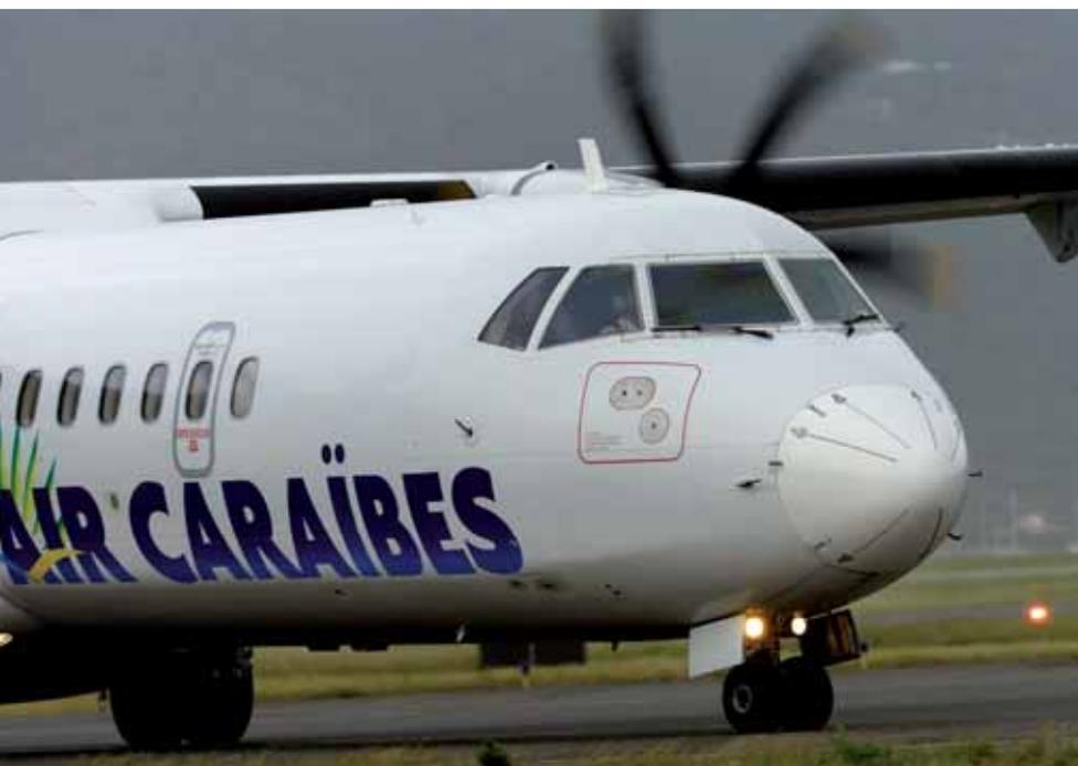
The ATR 42-500 and 72-500 are powered by the PW127E/F, utilising a six-bladed propeller. The ATR 42-500 has a 34-38 knot faster cruising speed than its -300/-320 counterpart variants. The six-bladed propeller lowers specific fuel consumption and noise emissions.
