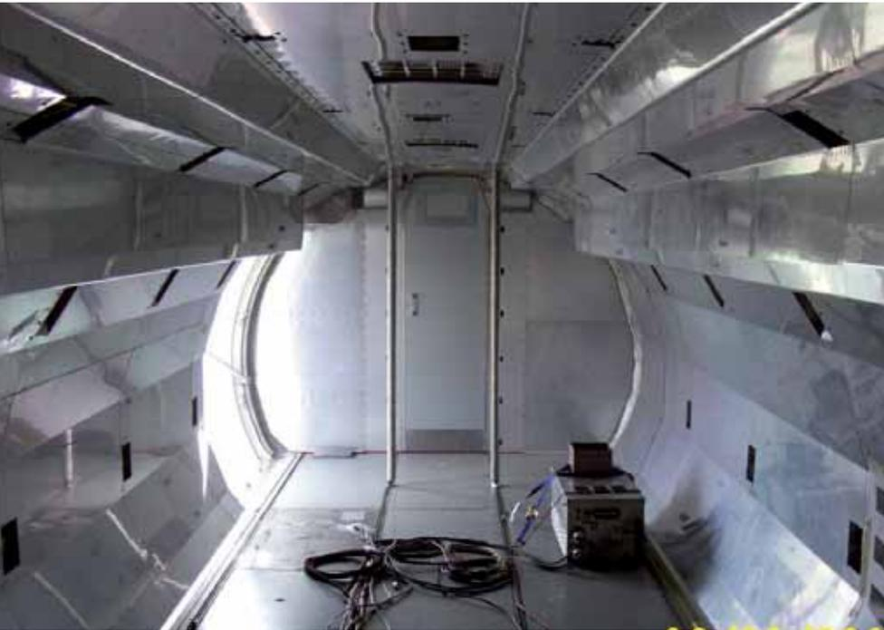
*Once converted to freighter, the fuselage interior is strengthened and lined to provide protection during container loading and off-loading.*
