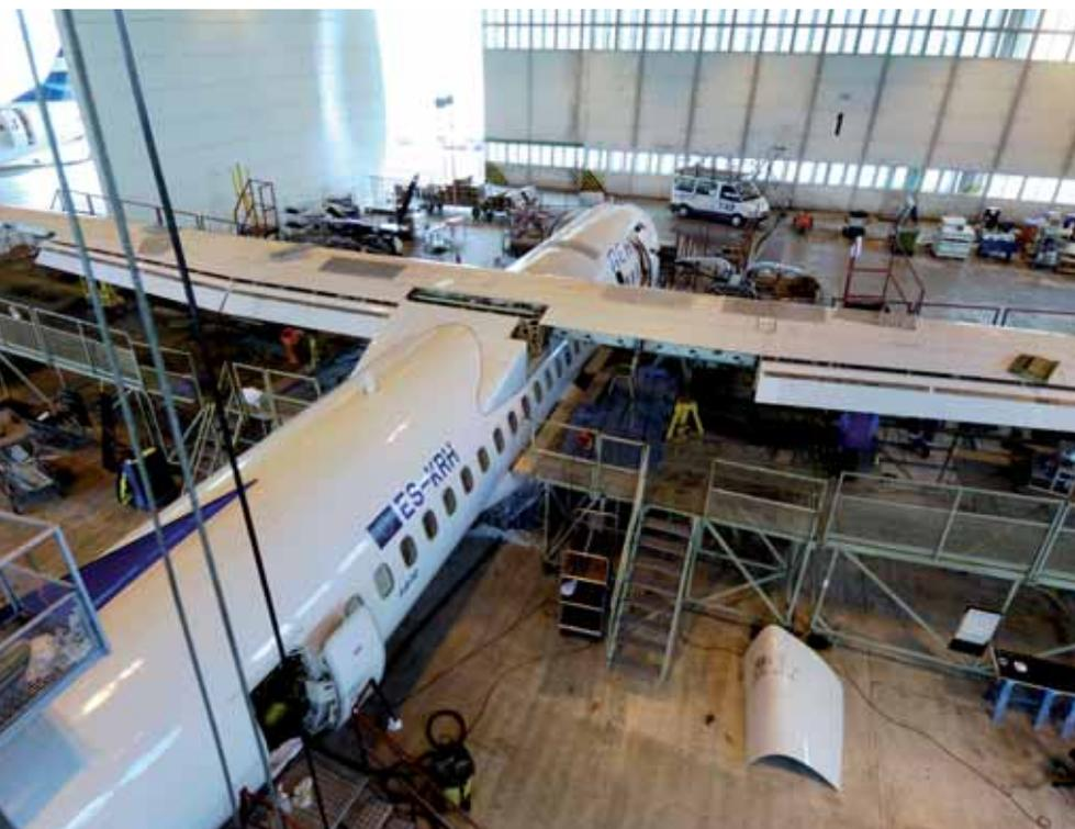
*The ATR 42's & 72's base maintenance programme comprises three major portions of system, FC-fatigue and calendar-fatigue tasks. Despite the aircraft operating on average cycle times of less than one hour, inputs for base checks result in maintenance reserves of less than \$100 per FH.*
