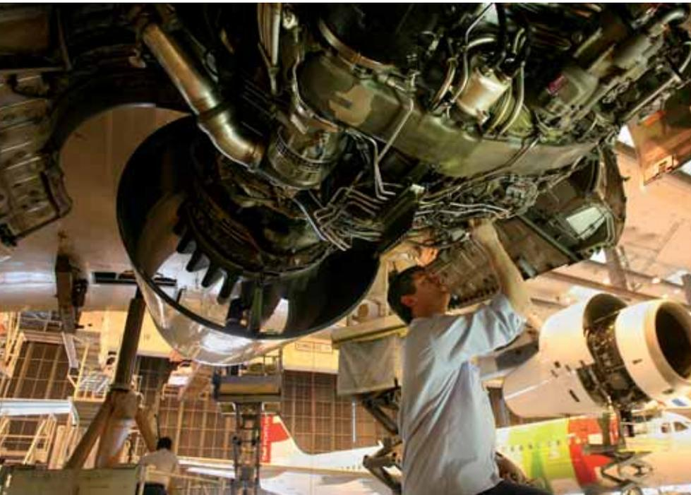
2,500MH. Non-routine work adds a further 4,500MH, including some cabin cosmetic items, while other items add 1,350MH. This takes the total for a C2 check to the region of 8,300MH.” This total is similar for the C6 check. Totals for the C1, C3, C5 and C7 checks will be about 7,800MH for aircraft in their second base check cycle.
