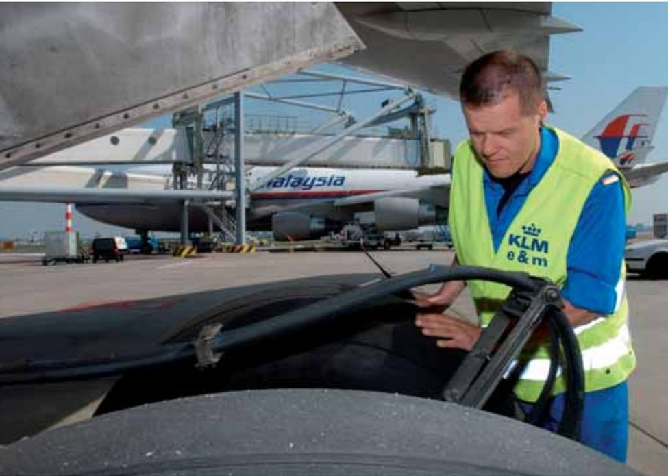
*Items such as brake disc thicknesses have to be monitored so that removal for repair and overhaul can be anticipated and planned at convenient checks, such as a daily or weekly check.*
