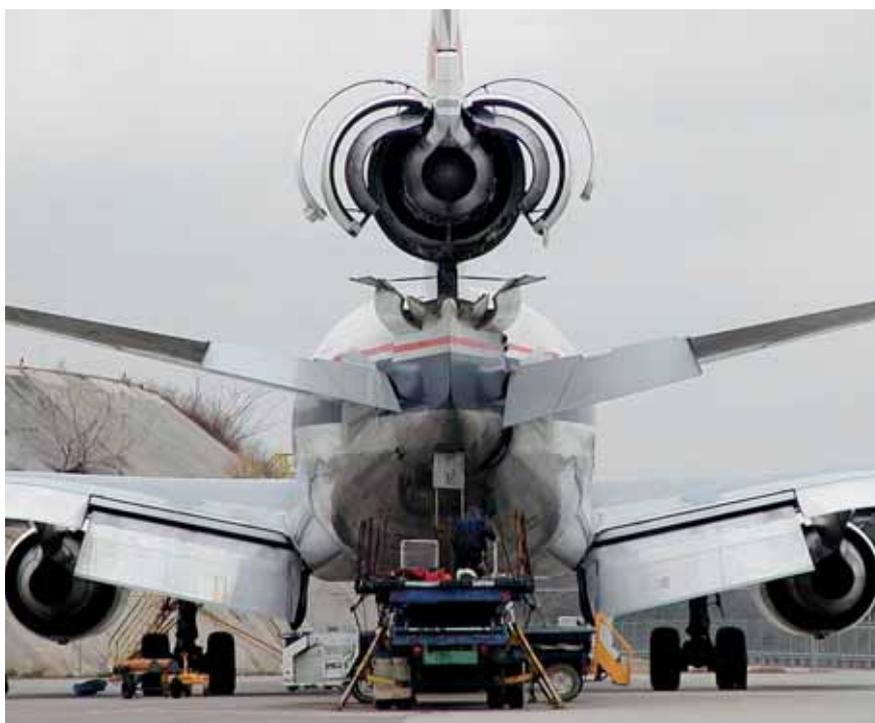
*The Phase III programme was initially introduced in 1992 to address performance shortfalls of some MD-11 operations. The Phase III modification was subsequently used on the whole PW4000-94 fleet. The main features of the modification were improved fuel burn performance and increased EGT margin. About 950 of 1,100 Phase I engines have been modified.*
