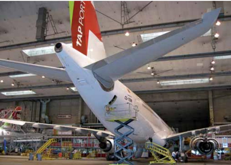
Total inputs for the cycle of eight base checks will consume 80,000-90,000MH and incur a total cost of \$4.7-6.0 million. Consumption will be lower for aircraft operated on medium-haul operations, but reserves per FH will be higher than for long-haul aircraft.
