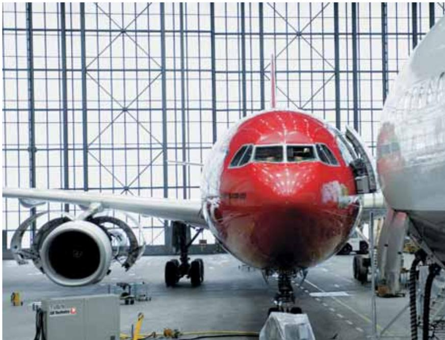
*Heavy maintenance visit worksopes will include routine inspections, non-routine rectifications, ADs & SBs, removal and replacement of rotatable components, customer items, interior cleaning and refurbishment, and stripping & repainting.*
