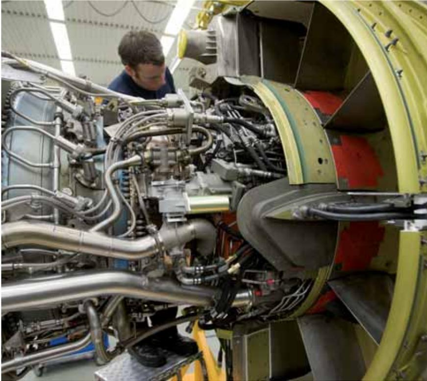
*Engine removals for shop visits will be a compromise between on-wing life that is possible with EGT margin and LLP limits. The workscope required on the HP modules, LPT and fan/LPC will depend on the utilisation of LLP lives and the subsequent removal interval that will be possible with the restored EGT margin.*
