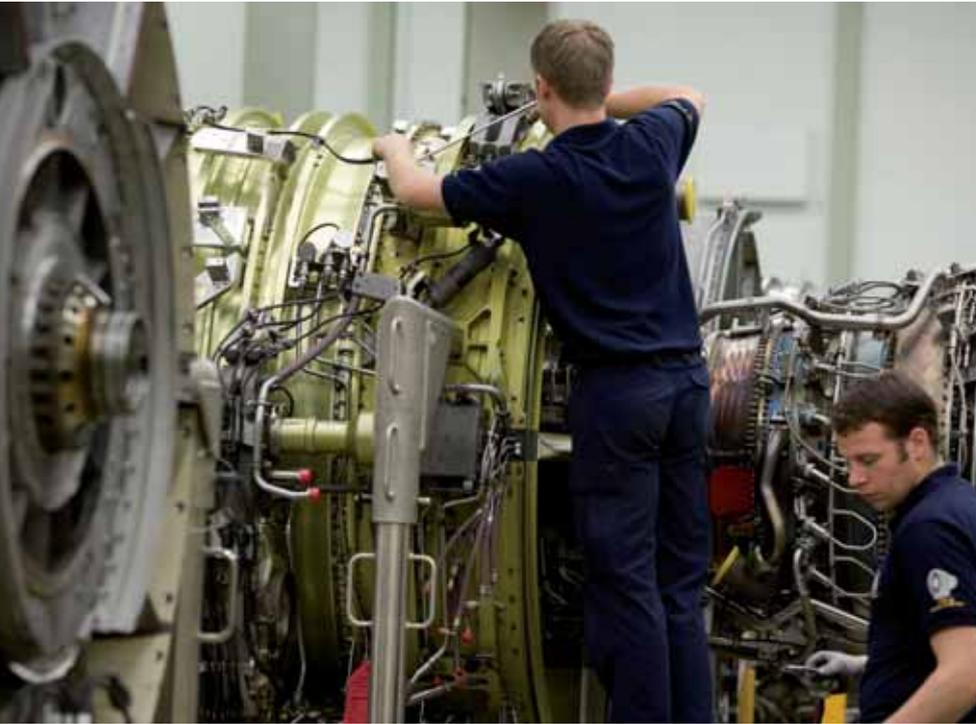
*Shop visit removal intervals for lower rated -7B variants are rarely due to EGT margin erosion. Engines can usually remain on-wing to the first LLP life limit.*
