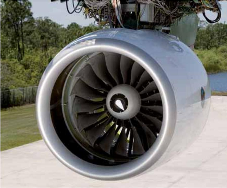
*Pratt & Whitney's GTF will have a bypass ratio of up to 10:1. This is made possible because the gearbox allows the LPT shaft to turn three times faster than the fan. The LPT consequently generates more power than it would in a conventional engine, and so can turn a larger fan.*
