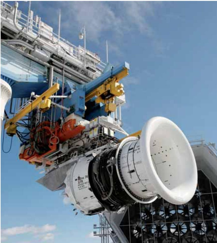
*The GenX is an enhanced conventional two-shaft turbofan that will have bypass ratio of up to 9:1 and an overall pressure ratio of 40:1.*
