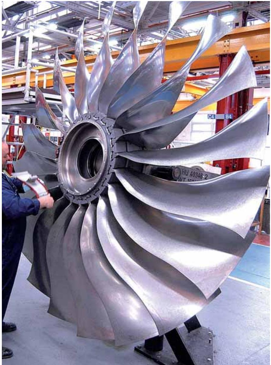
wide-chord, swept fan blades. This makes the fan more efficient than on current generation engines. The Trent 1000 will have 20 fan blades, and the Trent XWB will have 22 blades, compared to the Trent 700's 26 blades. The Trent 1000 and XWB models are also expected to have NOx emissions that are 35-40% within CAEP IV standards.
