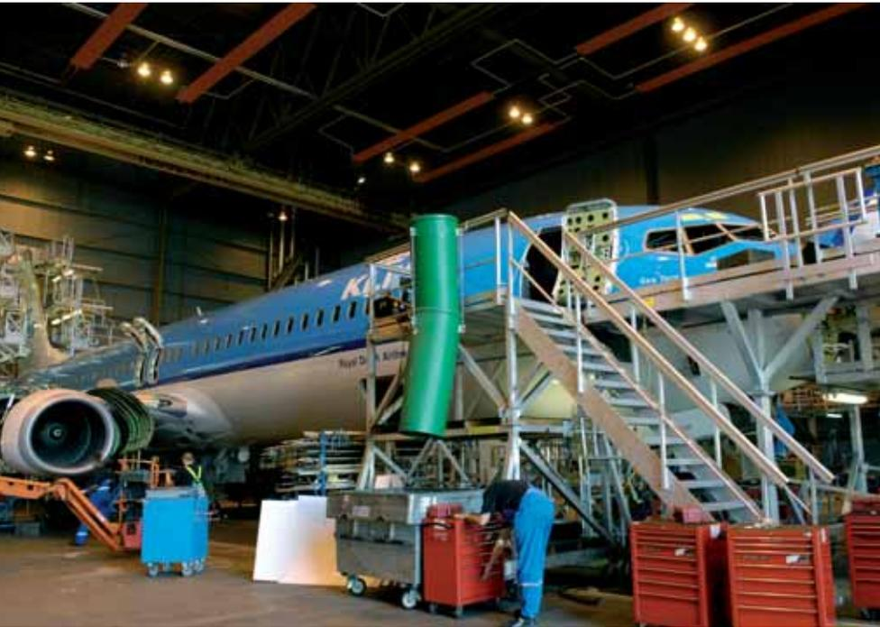
Base check workscopes include all the items the base checks of previous generation aircraft had. Unlike older generation aircraft, refurbishment of the interior is often treated as an on-condition item, rather than being performed during a heavy check.
