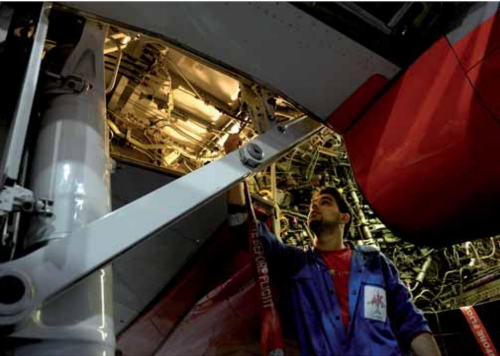
*The 737NG's maintenance programme consists of about 1,000 tasks. These have intervals specified in FH, FC, calendar time, or a combination of two of these criteria. Operators are free to group these tasks into checks in accordance with their annual utilisations and FH:FC ratio.*
