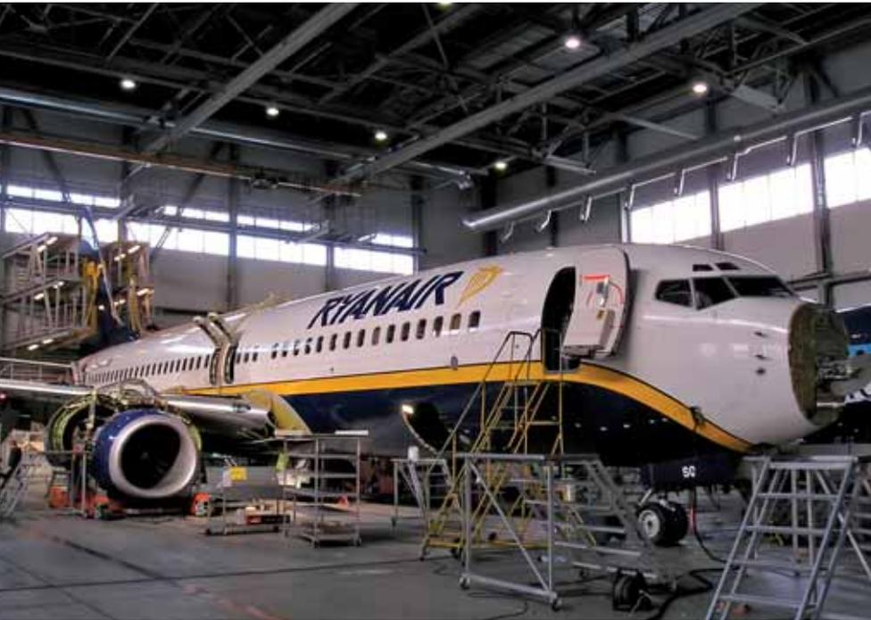
*The 737NG's flexible maintenance programme means tasks are not performed before necessary with the result that costs per FH for base checks are low relative to similar-sized aircraft types.*
