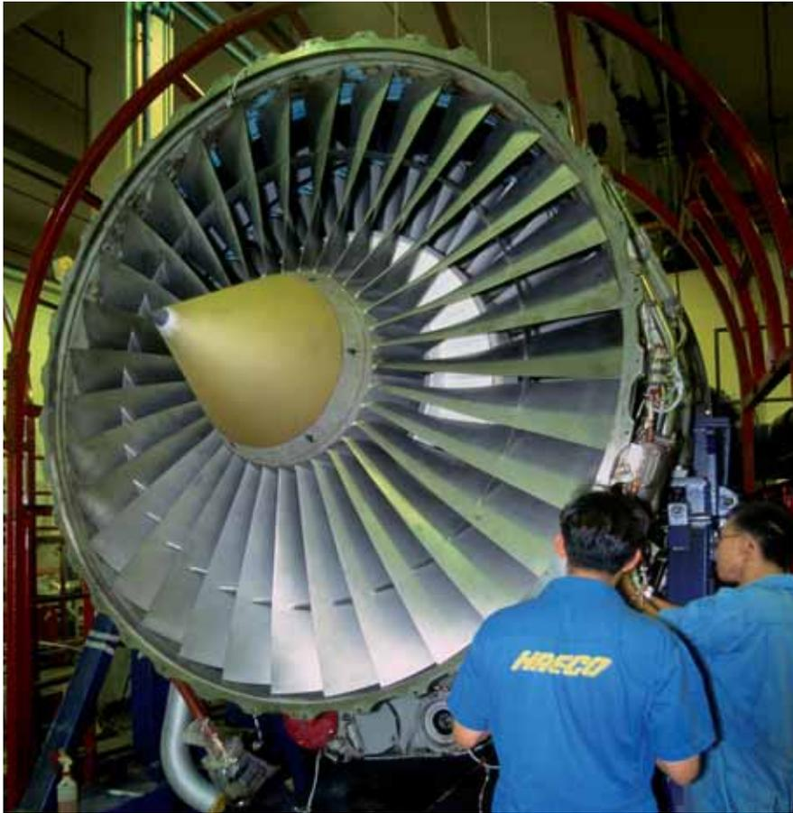
*The Rolls-Royce engine maintenance plan requires level 3 or level 4 workscopes on all engine modules at scheduled shop visits. This puts the cost of shop visit inputs at a high level relative to other engine types.*
