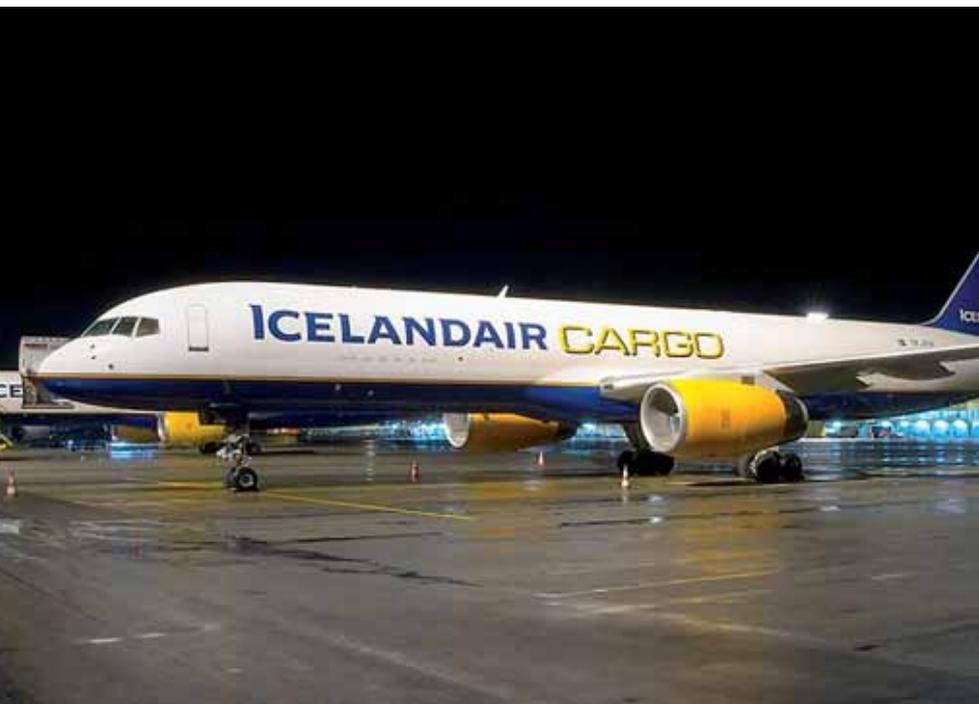
There are 400 RB211-equipped and 285 PW2000-equipped 757-200s in passenger configuration that are potentially available for conversion to freighter, of which 670 are above line number 210. These could have the second, third and fourth payload options.
