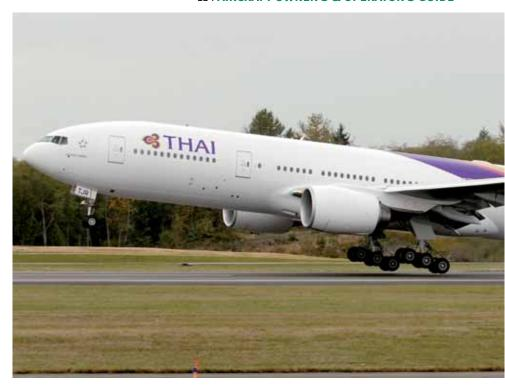
GE developed the GE90-115 for the 777-300ER and de-rated the engine design for the -200LR and 777F. Developments included aspects that improve fuel efficiency, thrust and the noise levels of the engines. The improved combustor means that the engine is producing no more than 50% of the carbon dioxide levels currently allowed by international standards.
