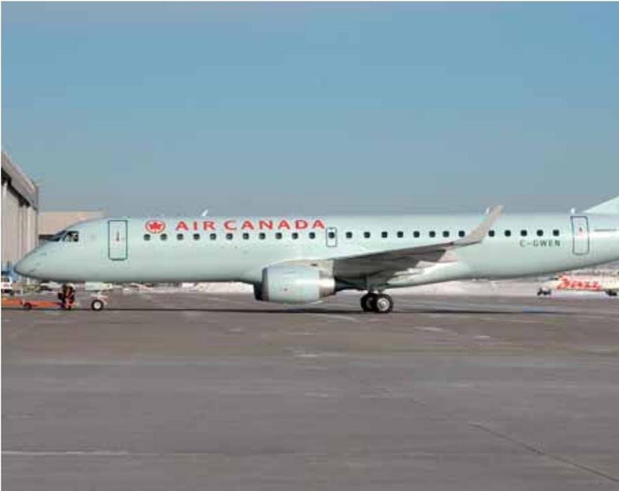
175 are powered by the General Electric (GE) CF34-8E, which has a bypass ratio of 5.0:1. The E-190/-195 are powered by the CF34-10E, which has a higher bypass ratio of 5.4:1. These bypass ratios affect the aircraft's fuel burn efficiency. The large RJ programmes that have been launched in the past two years use engines with higher bypass ratios than the CF34-8E and -10E. This clearly gives the new generation aircraft an advantage in fuel burn performance over the E-Jets.
