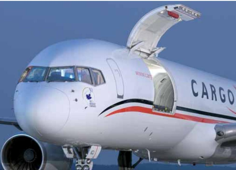
container/pallet positions. This gives the aircraft 6,600 cubic feet of maindeck cargo volume, in addition to another 1,790 cubic feet of underfloor space. This takes the total volume to 8,390 cubic feet.
