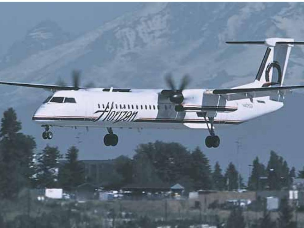
further success of the modern turboprop aircraft, and route density, a larger Q Series was needed. This variant is a further stretch of the fuselage by nearly 35 feet, compared to the Q100/Q200, and 23 feet compared to the Q300. This allows the Q400 to carry 69-80 passengers. The aircraft first entered service in 2000 with SAS Commuter of Scandinavia. The highest MTOW is 65,200lbs.
