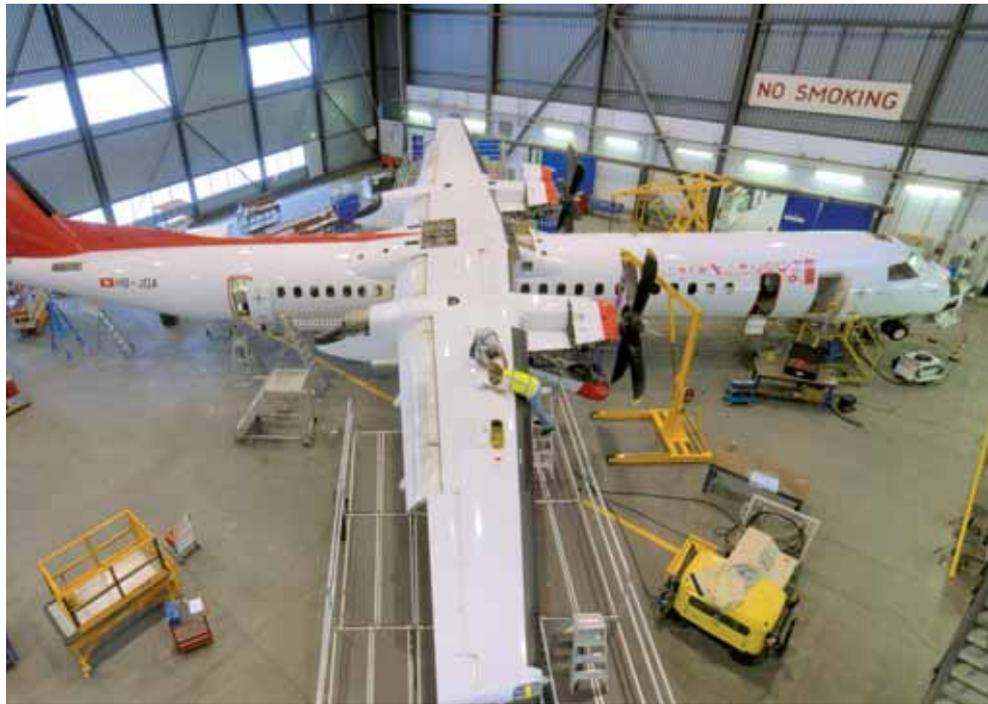
"We have equalised our A checks, so we have smaller checks at a shorter interval. These smaller packages can be done in an overnight check," says Kontorradvis.
