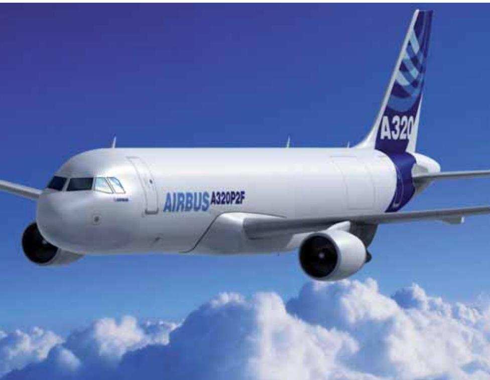
The A320F has a gross structural payload of 46,525-49,823lbs. This puts it between the 737-400 and 757-200, and close to the 727-200.
