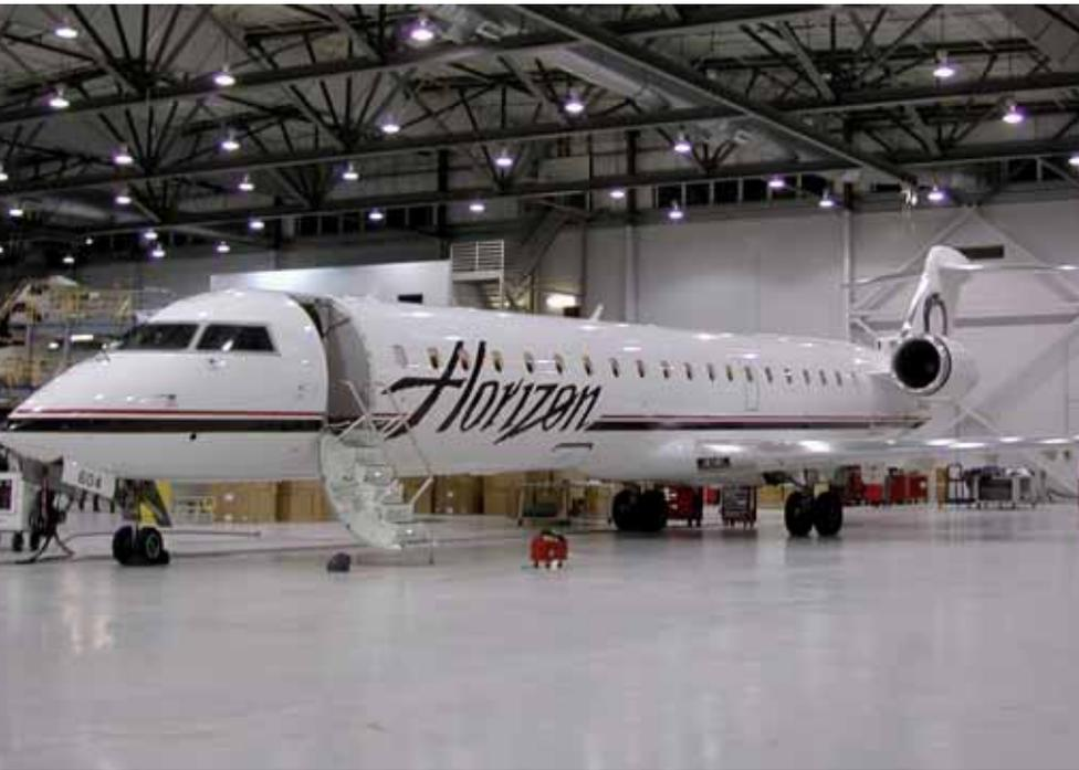
The current basic interval for the CRJ-700/900 is 4,000FH. Base check tasks and reserves are similar to the CRJ-100/200. The basic interval for the CRJ-700/900 will be extended to 6,000FH, and should have the effect of reducing base check reserves.
