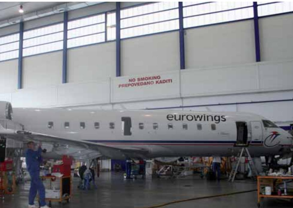
The CRJ-100/-200 have C check tasks with an interval at multiples of 5,000FH. It is simplest to have base checks every two years. Most out-of-phase & calendar tasks can be planned into base checks, even though their full intervals sometimes do not get fully utilised.
