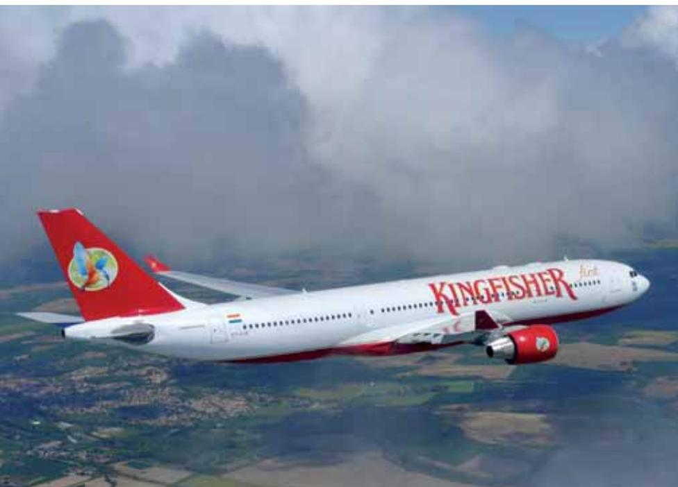
*The PW4000-100 powering the A330 family and the -112 series powering the 777 family have had similar success. Pratt & Whitney recently launched a new variant; the PW4170. This has a higher take-off thrust rating and higher EGT margin than earlier variants.*
