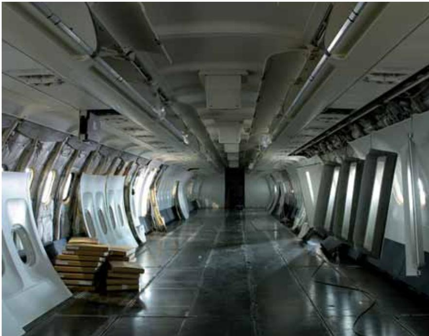
between each C check at 15-18 months. The C4 and C8 checks are heavy visits, and include structural inspections, and are performed every five to six years. The other six C checks are lighter.
