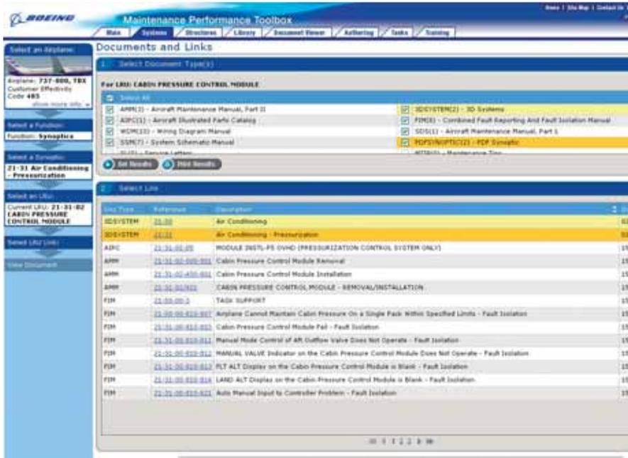
Documents can be made available on-line to technicians and mechanics almost instantly. Another improvement is that technicians and mechanics do not have to spend a lot of time searching printed manuals for instructions and parts catalogues. With the right equipment and technology, relevant pages can be found within seconds, and viewed on screen. Mechanics also make fewer mistakes, and always have access to the most current approved technical information.
