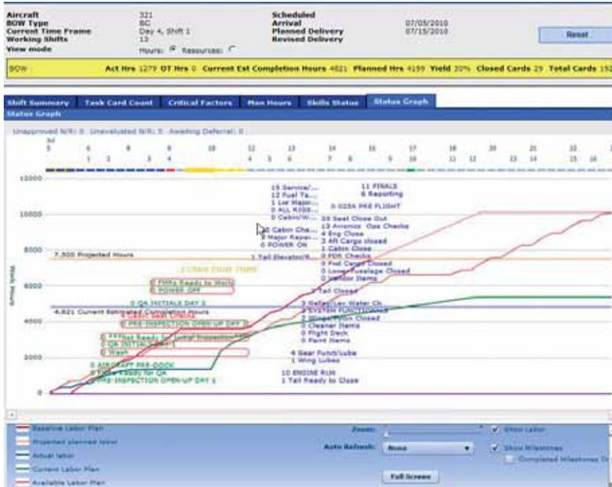
EmpowerMX's FleetCycle system has a status page used for monitoring the progress of a check. Colour-coded plots are used to indicate accumulated MH used, MH available and MH required to complete the check on time.
