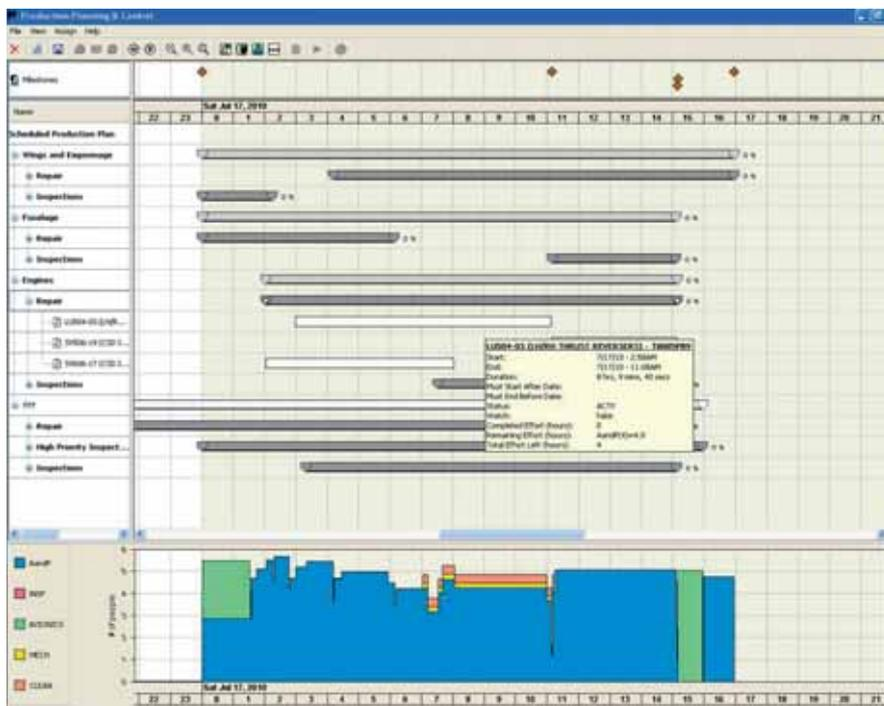
*MXi's Maintainix system plots a gantt chart for a planned check, using horizontal bars in the upper screen to denote tasks and task groups. A histogram in coloured bars in the lower screen denotes labour and labour skills required throughout the period of the check.*
