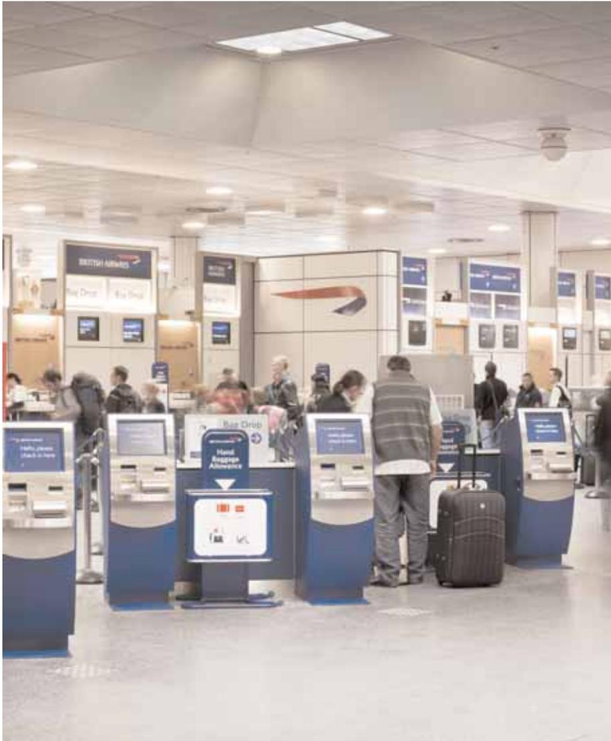
airports are both challenged to use less airport space and reduce passenger transit times, and automate the baggage check-in process. BagDrop's automated bag-drop process uses a bank of unmanned desks, and claims to increase an airline's check-in capacity by up to 80% through reduced processing time. The system also uses less overall space than the conventional system of manned desks.
