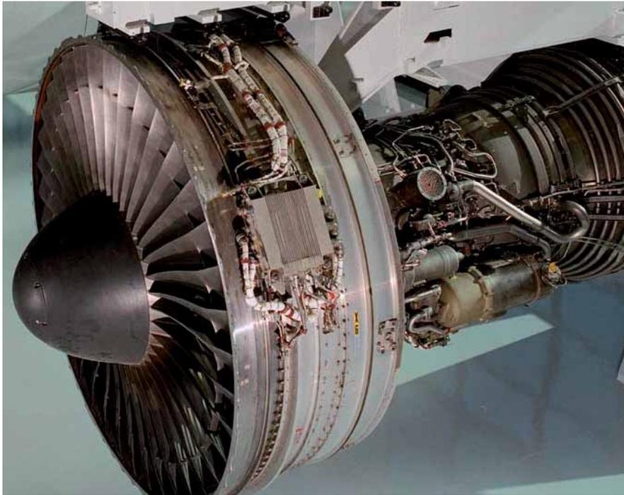
main engine control (MEC), fuel pump, pneumatic starter motor, variable stator vane actuators, and sensors.
