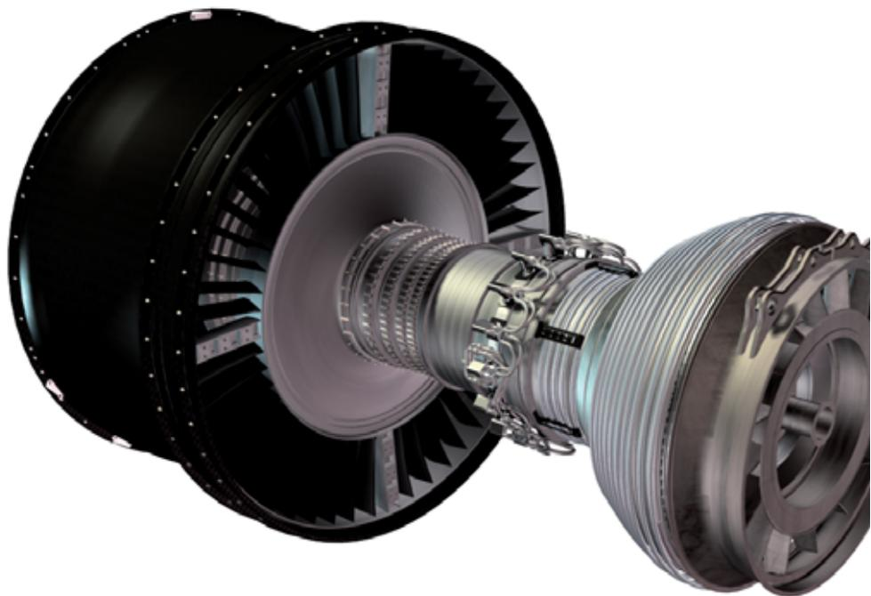
*The small diameter of the LEAP-X's core engine is illustrated by this computer representation of the engine, and demonstrates how the engine's bypass ratio of 12:1 will be achieved.*
