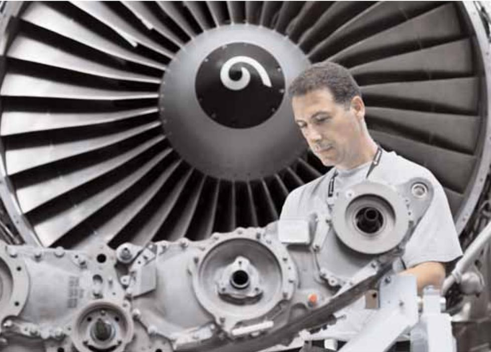
and Westfield Gage Company Overhaul & Repair, offer cleaning, repair and specialist coating of shafts, discs and rotating airseals.
