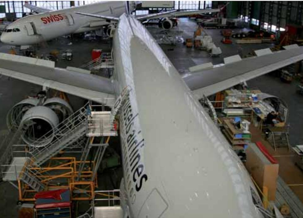
routine ratio steadily climbs during the first base check cycle, and continues into the second base cycle. Non-routine ratio is partly influenced by corrosion and structural fatigue. Checks with a high level of access for deeper inspections tend to have high non-routine ratios.
