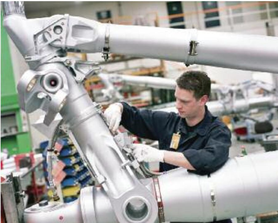
corrosion. “Preventative maintenance is performed on the components on the landing gear that are maintained on an on-condition basis,” says Tielman. “The first action after the stripping of paint is to inspect for corrosion. Some non-destructive tests (NDT) are carried out at this stage.”
