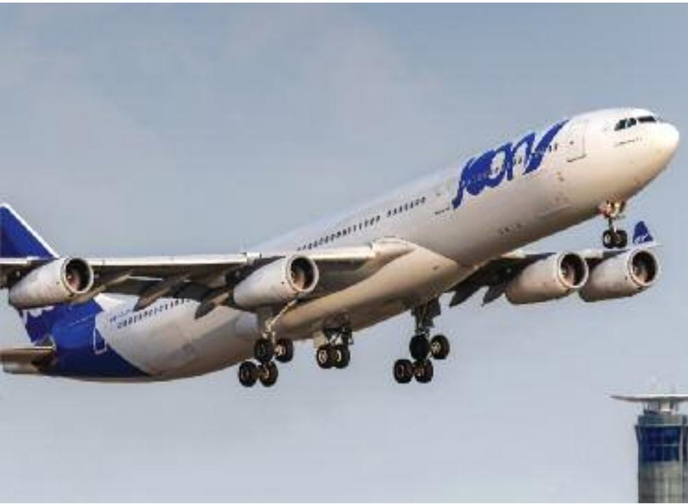
The -5C is the highest-rated of all CFM56 family engines, and like the -3 series the -5C is particularly sensitive to EGT margin and performance erosion. Recovered EGT margins following an SV are 35-40 degrees for the -5C4 variant, and about 60 degrees for -5C2 engines. This allows mature removal intervals of about 10,000 engine flight hours (EFH) for the -5C4 and up to 14,000EFH for the lower rated -5C3 and -5C2 when they are operated at about 7.0 EFH per EFC.
