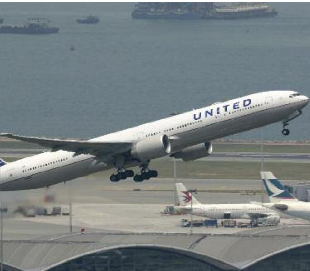
*The 777-300ER is a prime example of the benefits of twin-engined configuration and the economies of scale provided by a stretched fuselage. Its fuel burn per ASM is 14% lower than a 747-400 and 5% lower than the 77-200ER.*
