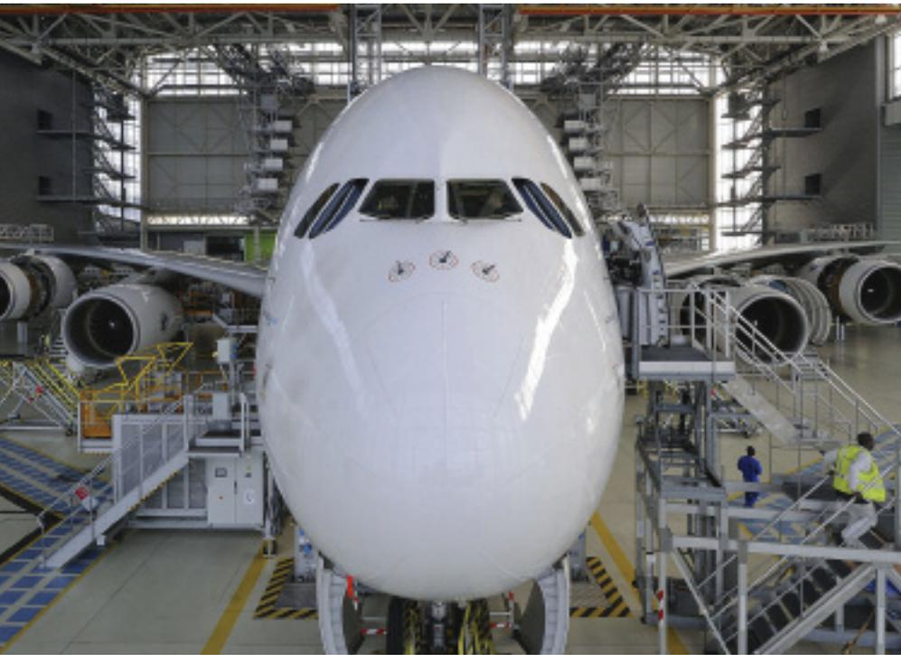
Lemaire. An airline that keeps a block system of arranging A checks could treat this as an 8A group of tasks, and perform it every eighth A check, which would be about once a year.” This group could be referred to as the 8A tasks, since their interval is eight times the 1A interval.
