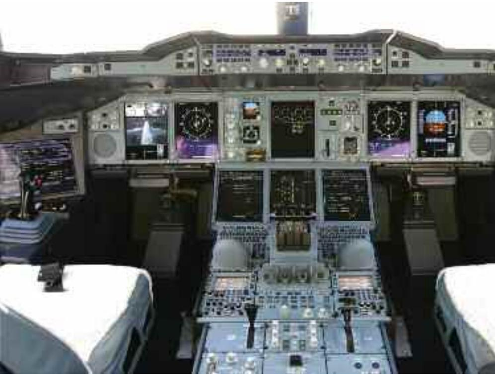
include the A380, A350, 787 and Bombardier CSeries, have on-board maintenance systems that further simplify the diagnosis of technical faults and flightdeck effects. This will reduce the aircraft's line maintenance requirements and improve technical dispatch reliability.
