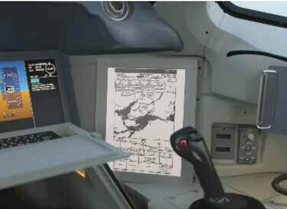
“It allows information to be shared between the pilots and mechanics electronically. The information is first entered by the pilots, via the OITs, and by cabin crew using their own system.
