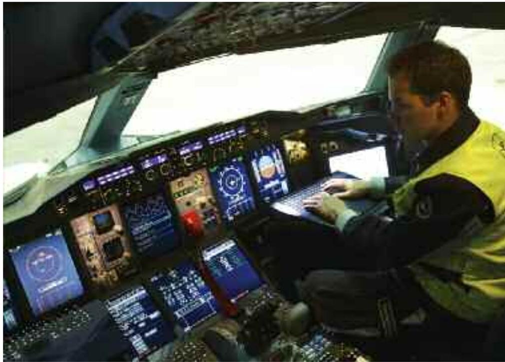
flight the CMS generates the PFR, which summarises all failure messages from the last flight leg. The report is stored on the aircraft server and sent to MCC via ACARS.
