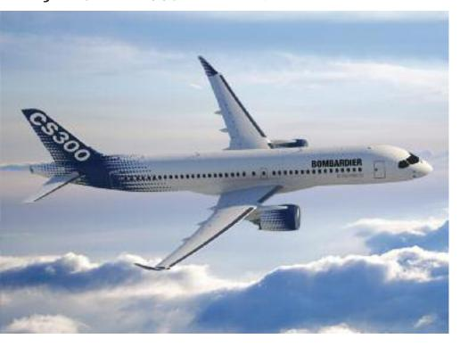
The CSeries will use the ultra high bypass PW1500G. This will give the two CSeries models a fuel burn advantage of about 20% over similar-sized current generation aircraft.
