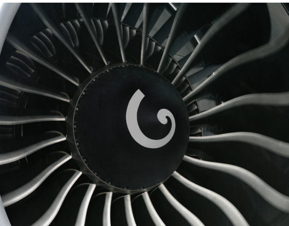
and thrust ratings of 76,000lbs to 93,700lbs (see table, page 5). Conceiving an engine that was capable of delivering this amount of thrust required the GE90 to have a higher overall pressure ratio than the CF6-80C2 and -80E1 families. The CF6-80E1 has an overall pressure ratio of 34.8:1.
