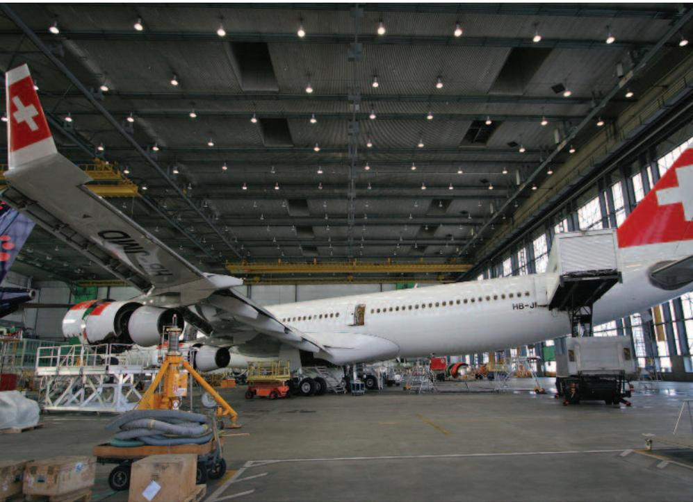
Aircraft systems are tested during airframe checks. This can reveal faults with rotables, which are then removed, repaired and replaced. The cost of this should nevertheless be regarded as a separate element of aircraft maintenance.
