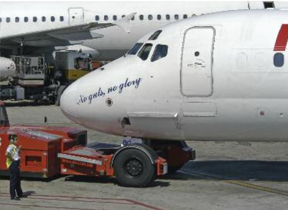
steering tiller on the flightdeck to make directional adjustments, as they would with a conventional taxi situation. These steering inputs turn the turret on the TaxiBot, which turns the wheels on the tug vehicle to steer in the required direction.
