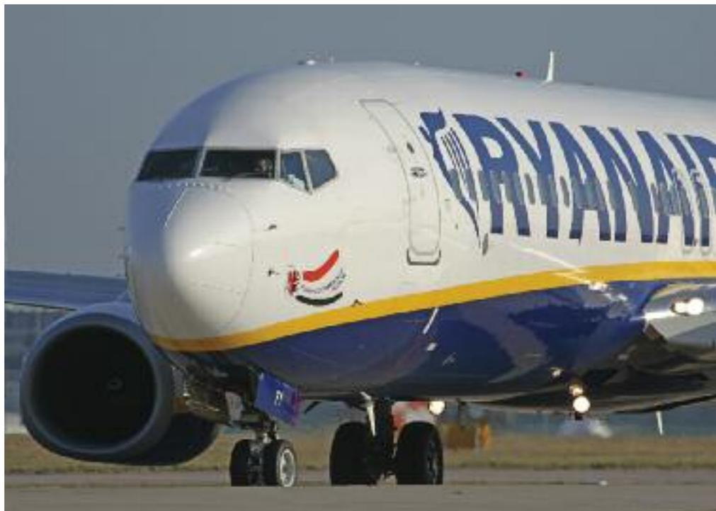
The majority of CFM56-7Bs are operated on 737-800s. The largest number of engines powering the 737-800 are the -7B26, -7B26/3, -7B26/E, and -7B27.
