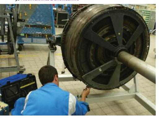
with a time-continued module that is in a better maintenance condition and has LLPs with longer lives; to put the module through a relatively light shop visit and replace those LLPs with the shortest lives; or put the module through a full shop visit and replace some of the LLPs, either with time-continued parts from the used market or with new parts.
