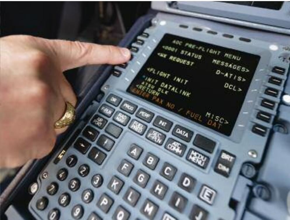
*ACARS messages are still the main method for sending and receiving data messages on the flightdeck. The number of connectivity systems that are available for making ACARS communications has increased, and transmission rates have also improved. ACARS messages are used for all types of flightdeck communications.*
