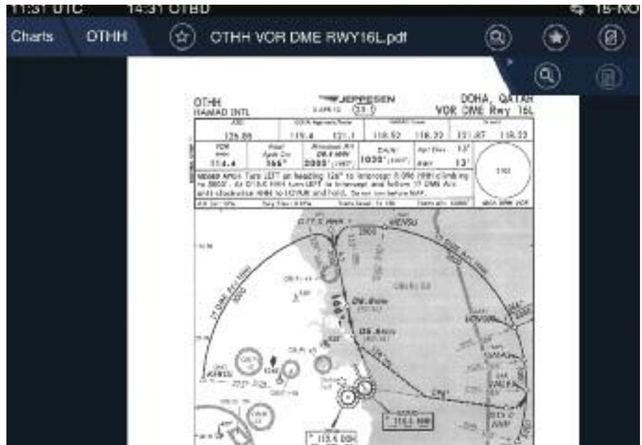
ASIG provides its flyTab® product for Class 2 EFB solutions using iPads. flyTab® includes a Software Developers Kit (SDK), mounting device, a power-conditioning module (PCM) and an Aircraft Interface Module (AIM), in addition to custom iOS applications development, and airframe integration services.
