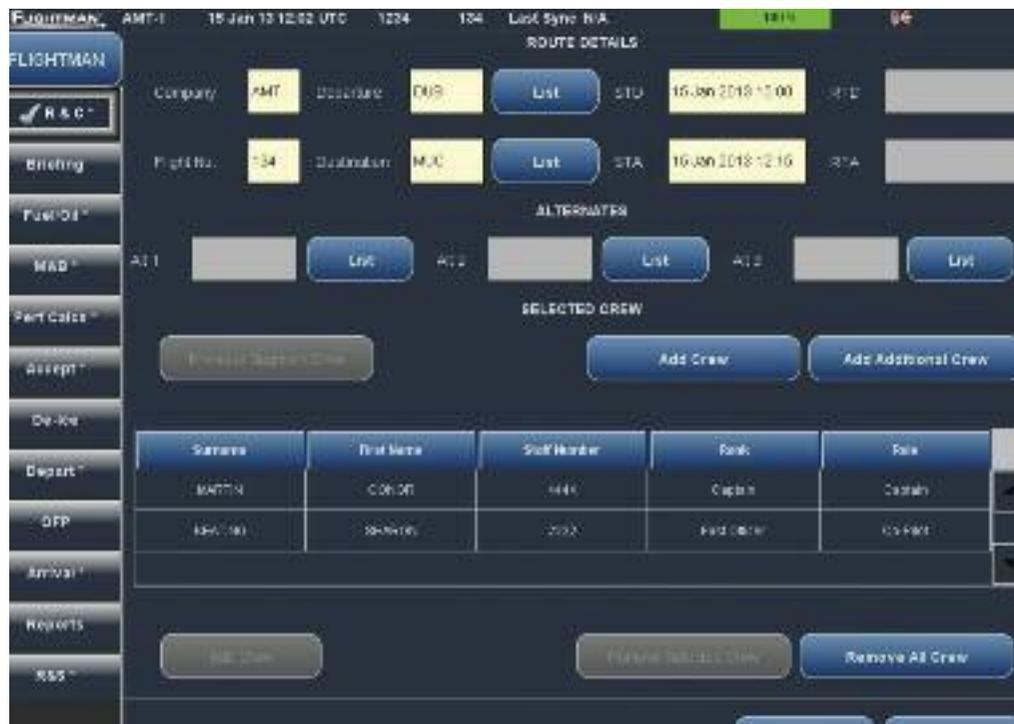
system is designed as a complete replacement for the aircraft paper technical log.
