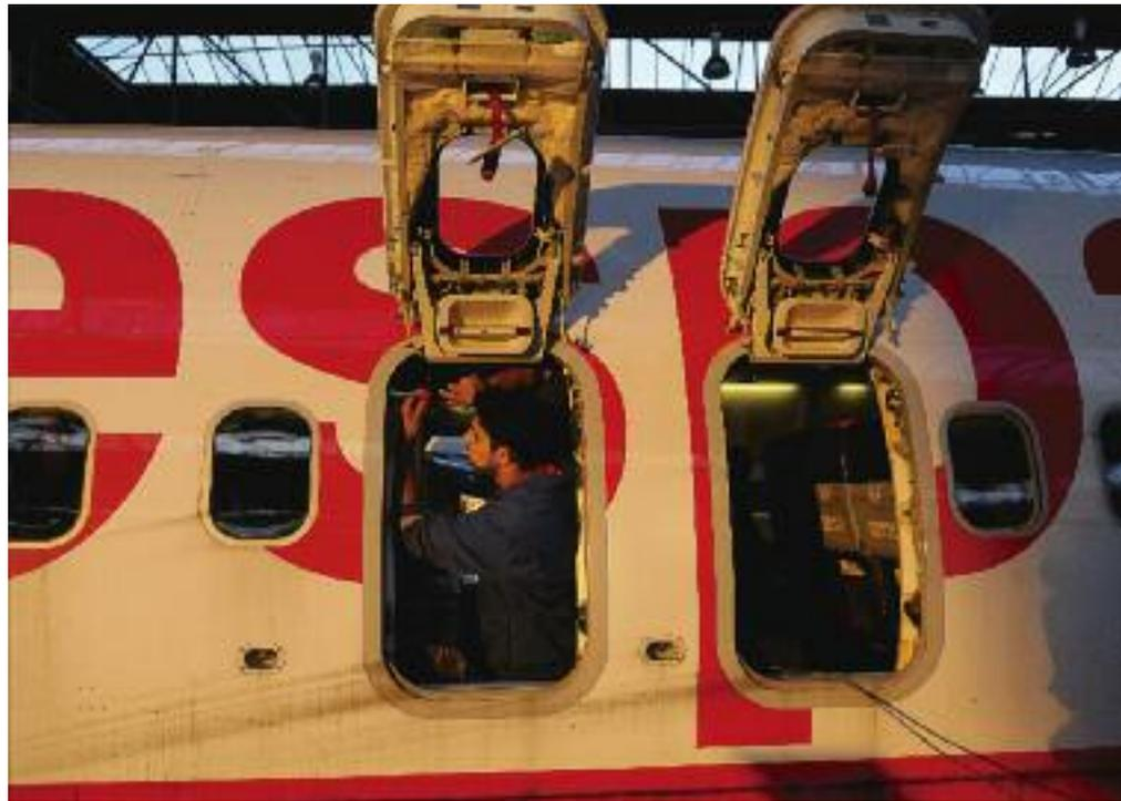
interval. According to the MPD, the actual inspections require only 4.50MH, but use several hundred MH for the removal and reinstallation to gain access.
