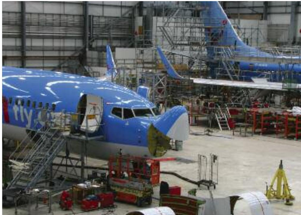
base check cycle will therefore be 21,000-22,000MH. This will be used over an actual interval of 10-11 years because of typical interval utilisations, even though the MPD interval is 12 years. This will therefore be equal to an MH consumption of 0.61-0.67MH per FH over the full cycle interval.
