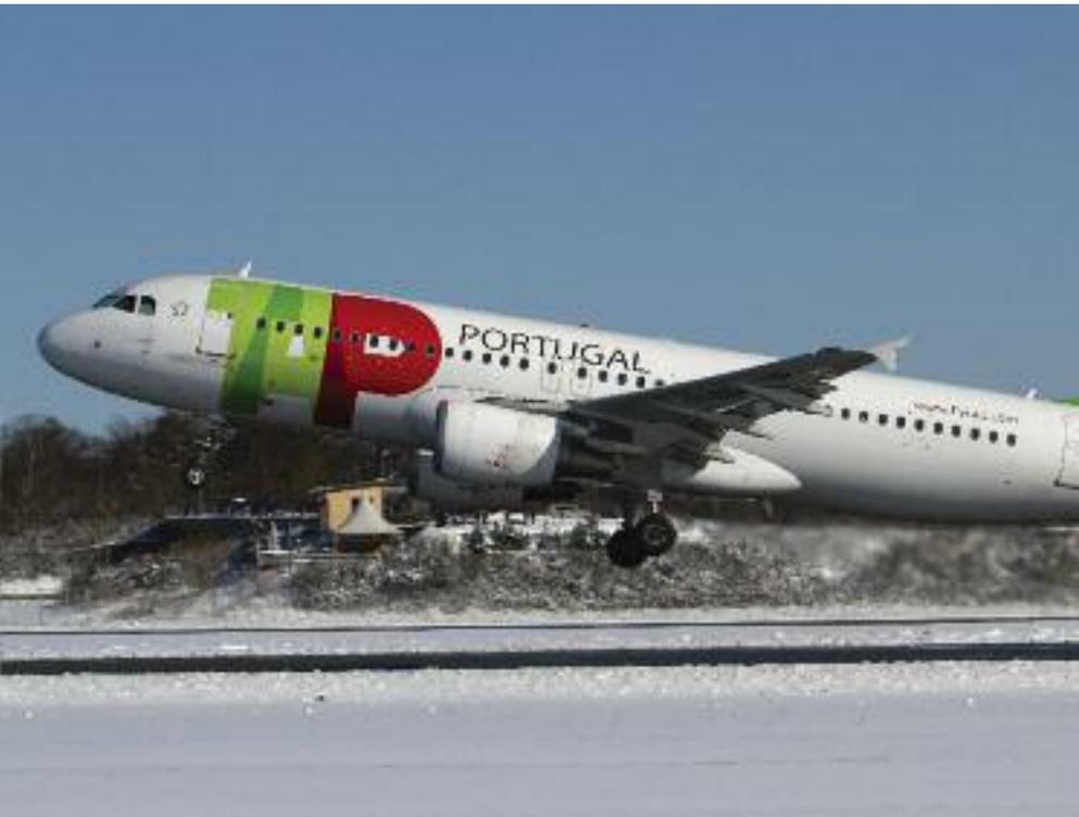
CFM-powered A320 TAP departing from a snowy airfield. Low OATS will help maximise TOW, allowing the highest de-rate to be applied.
