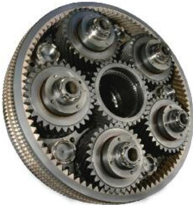
fixed oil pressure line into their shaft bearings that goes through a seal diaphragm to connect to the nacelle support vane. The outer ring gear is bolted to the fan hub and 2 sliding seals allow it to turn.
