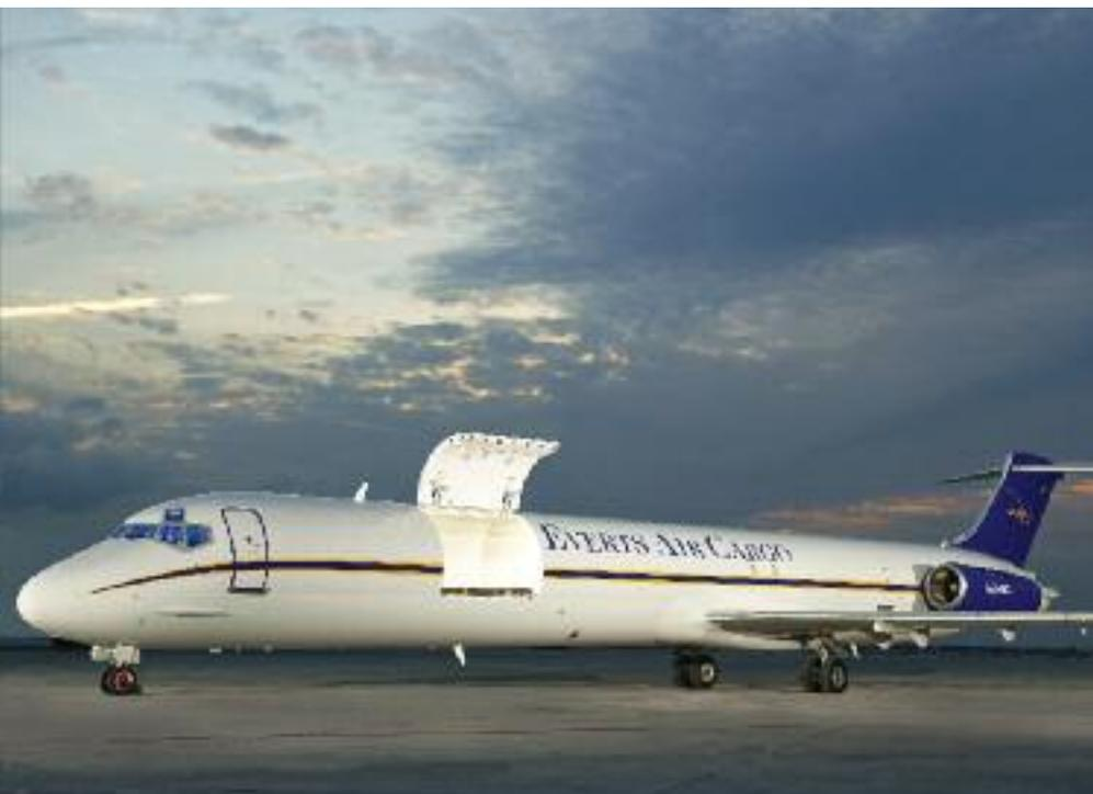
QC aircraft are fitted with a large cargo door, but maintain elements of their passenger cabin interiors such as the overhead luggage bins. This allows them to be quickly converted between passenger and cargo configurations.
