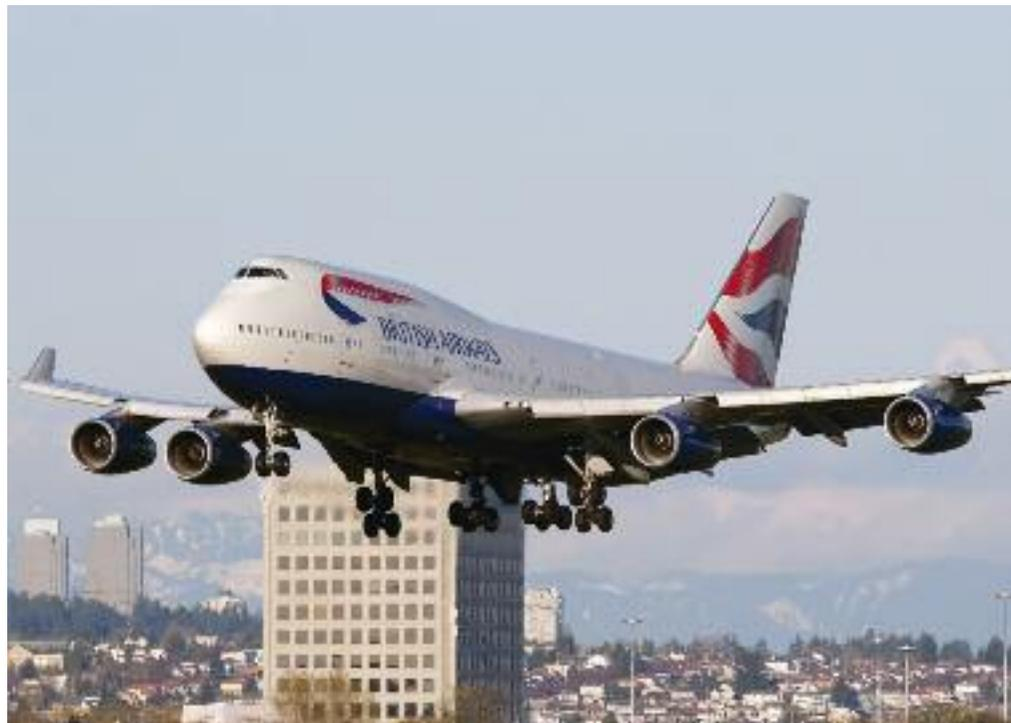
*The 747-400 is unable to compete with twin-aisle, twin-engine designs in terms of cash operating costs. This makes it a prime candidate for replacement. Large numbers have already been replaced by the 777-300ER.*
