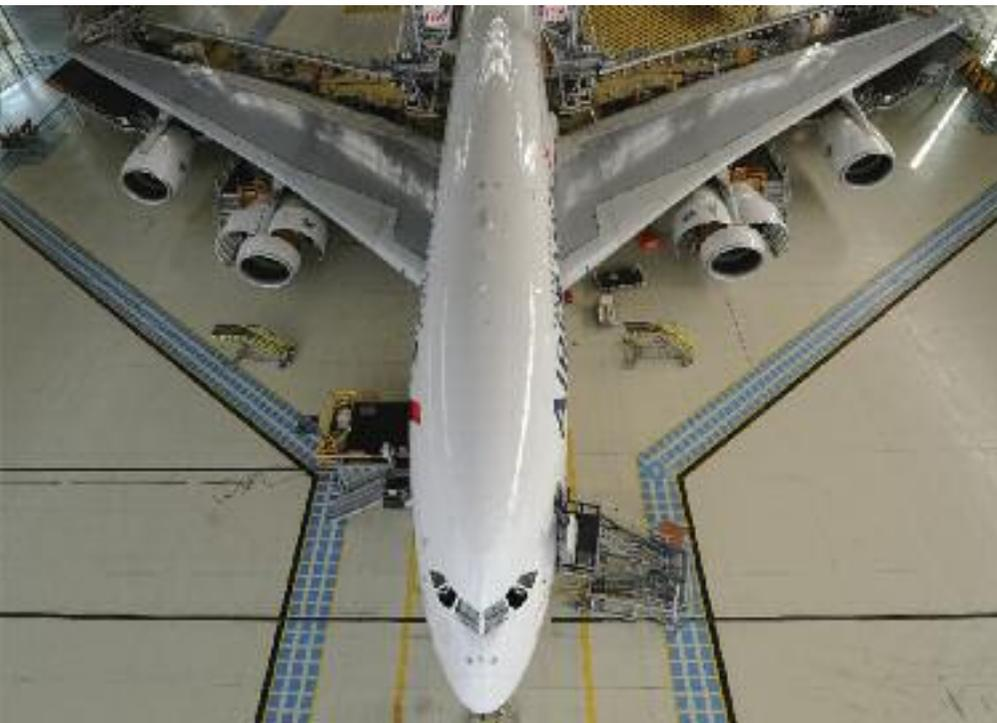
*The A380’s standard base check interval is 24 months. The base check programme is a system of six checks, with heavy maintenance visits at the third and sixth checks. The oldest aircraft have now been through their first heavy checks, the third in the cycle.*
