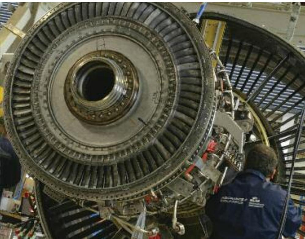
since new.” This life limit may compromise the engine’s optimal engine removal and shop visit pattern. Most engines affected by this AD have now had new P/Ns of the relevant LLP replaced.
